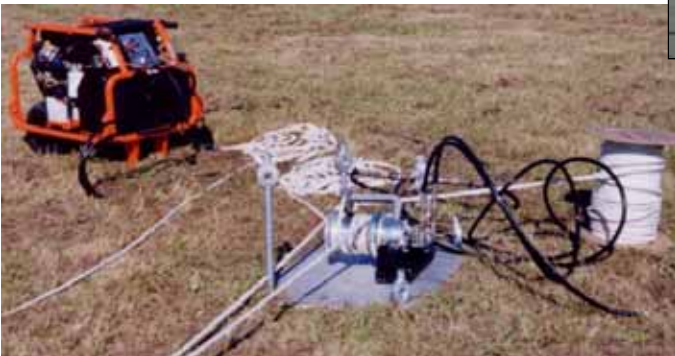
The Lindsey 7004 Capstan and Hydraulic Power Supply
