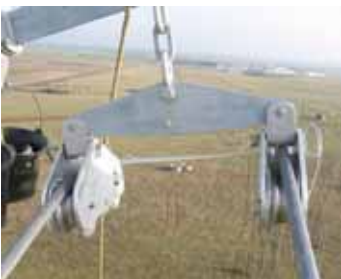
The 7060 Double Roller & Clamp eliminates the need to transfer conductors to clamps after stringing.
